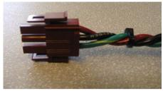
**Note:** If you are not using a Nortel-supplied PDU, have a qualified electrician connect the cable appropriately to your DC power plant. The 1002rp uses a negative 48 V power supply, therefore the red cable is negative (-48 V) and the black cable is the ground (GND).
